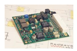
The PS140 provides 4 regulated voltages: +5, +12, +12 and -12 V. It also has a 3 A integrated battery charger and "hot plug" capability.
