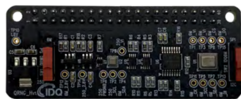
Evaluation board for IDQ250C2/IDQ6MC1
